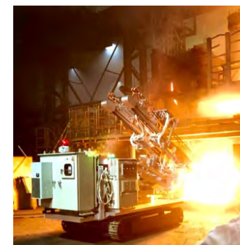
A radio-controlled robot that is involved in the furnace operation
