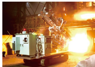
Wireless robot for measuring the temperature of molten steel (Yamaguchi Division)
