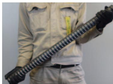
USD685B D51 ultrahigh-tensile threaded rebar
