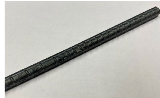
Success in trial rolling of 10mm rebar
